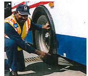
Wheel devices push whatever is caught out of the path of the bus.
